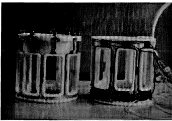
Fig 1: 8-channel phased array coils; Figure 2, Example of SNR Measurement circles on an one channel image using Collected using 8 channel neonate phased array.
